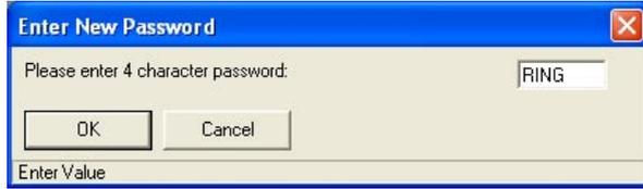
A new marSetup password cannot be entered until the current password has been read from the exchange.
