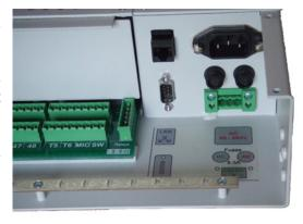
A serial printer can be connected to the nanoSwitch. The wiring for the port is the same as on a Personal Computer. The manual for the printer will give the required wiring and connections. The serial printer is set up as 115200 baud, 8-bits and 1 stop bit and CTS/RTS handshaking.
