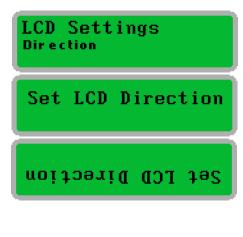
LCD display, when the system is installed in a rack or on a bulkhead.
